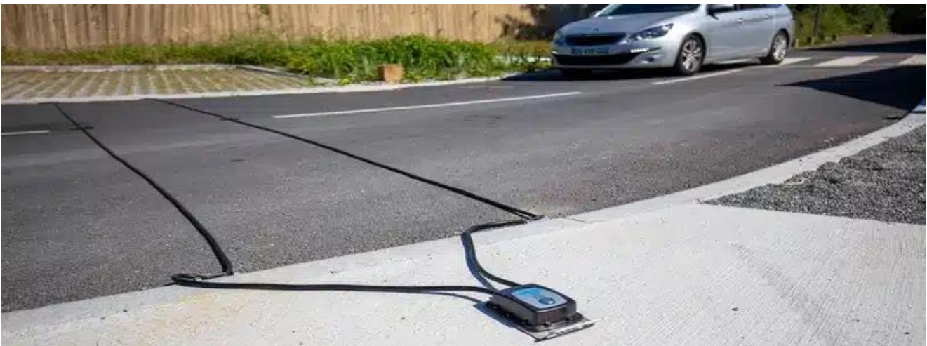
Figure 5. (Orbital Geospatial Services, 2024, Pneumatic Road Tubes or traffic counters for traffic surveys)
